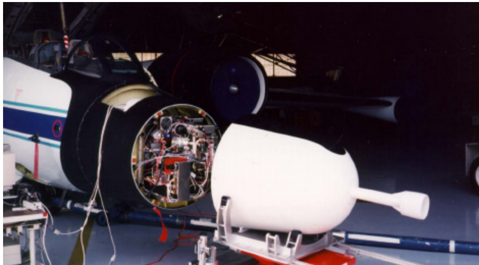
Figure 1. The PALMS instrument loaded into the nose of the WB-57 aircraft.
